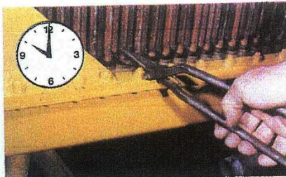
Hand tool dislodges tube from locking seal.
